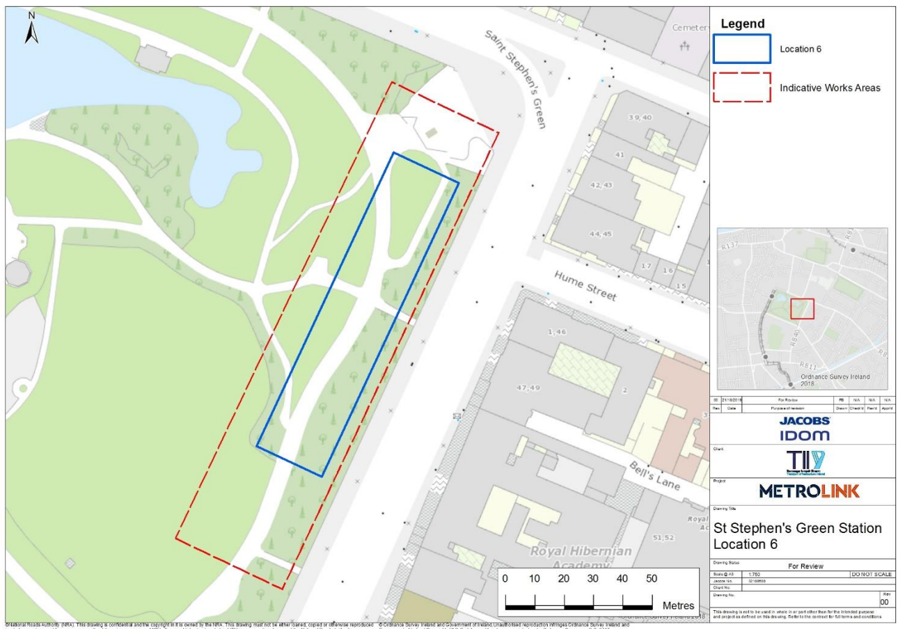
Figure 6.6: Location 6 Station box and indicative construction zone
